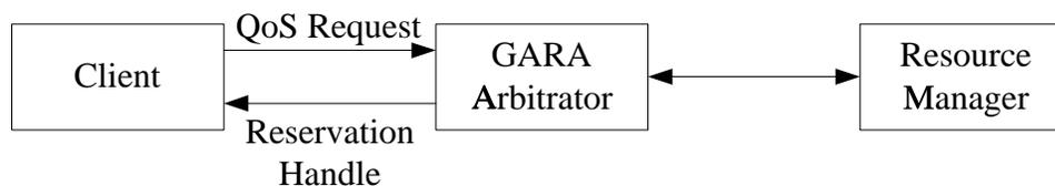
Figure 4.1: A program makes requests to the GARA Arbitrator which mediates access to the resource manager. If a reservation can be made, the GARA arbitrator returns a *reservation handle* describing the reservation.
